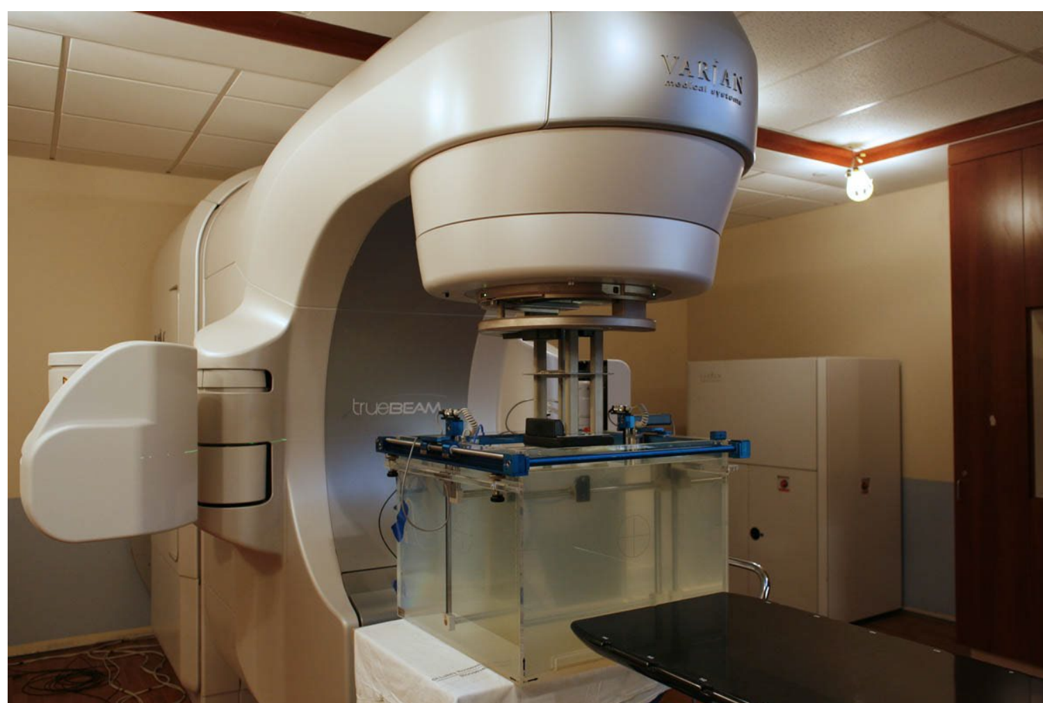
Figure 1: Varian TrueBeam linear accelerator with the Scanditronix-Wellhofer phantom positioned for data collection
